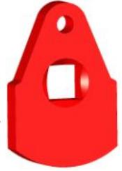
Now convention says that the right hand side should lead. All this means is that when the model is running forward, the right hand crank is 90 degrees, or a quarter of a revolution in front of the left; hence the term 'quartering'. We always observe this rule of the right hand side leading, though it would make no difference at all to the running if it were the other way round.
