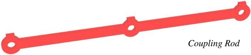
There are two coupling rods. These are the rods that have three holes in them, and their purpose is to link the three pairs of wheels together.
