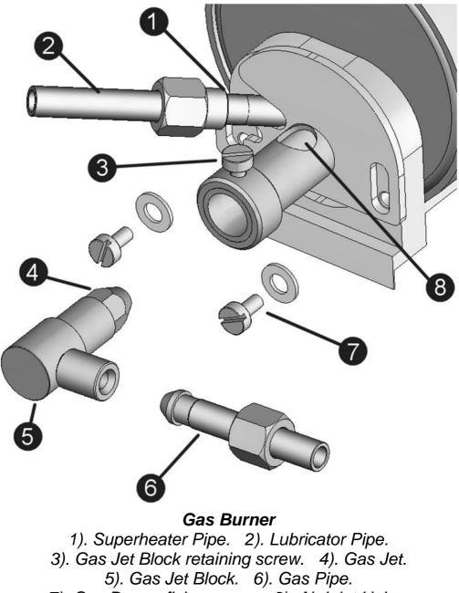
7). Gas Burner fixing screw. 8). Air Inlet Holes.
