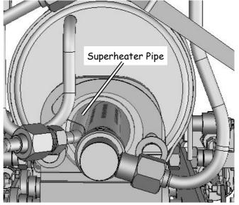
mounting flange to allow the superheater to pass through it. Ensure that the superheater is well over to the left hand side of the flue tube for its full length (see drawing on previous page).
