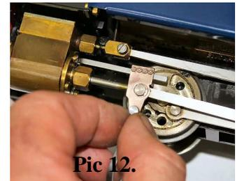
5/ If fitting the SBCHC kit, the dummy combination lever can now be connected.
