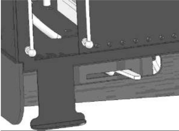
*On a manually operated Silver Lady, the lever to operate the Dummy Drain cocks / Exhaust Valve, protrudes through the chassis frame, under the Right Hand cab floor. The drawing opposite shows the valve set for 'Exhaust'.*
