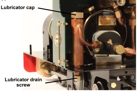
Replace the cap. Take time filling the lubricator, especially when cold, as the oil takes time to run down and may trap an air bubble. Both cap and drain screw are fitted with '0' rings and need only be closed finger tight.
