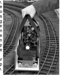
Because the loco wheels sit in cut -outs in the base, it is necessary to lift the model very slightly as it wheeled along. Once wheels are clear of the cut-outs. they will roll along the base. Hold the cradle base while rolling the loco along to prevent it from sliding. Do not lift the model by holding the sides of the bunkers, always hold the footplates.
