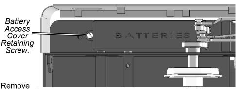
the cover by unscrewing the retaining screw at the rear of the cover. The Left-hand side of the cover can then be eased out. Slide the cover to the left and remove it.
