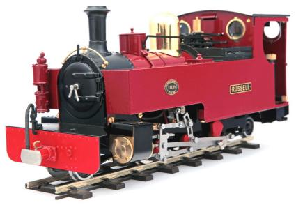
'Russell' is based on the well known 2-6-2 tank locomotive still running today on the Welsh Highland Railway in North Wales. Built by The Hunslet Engine Co. Ltd. of Leeds in 1906, it has undergone a number of changes over the years and the model depicts it as running in the early 1920's and as it currently appears.
