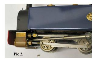
2/ Fit the slide bar by passing the two screws you have just removed, through the holes in the curved part of the slide bar and into the cylinder block as shown in Pic 3. Nip up but do not tighten at this stage.
