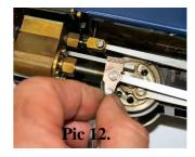
5/ If fitting the SBCHC kit, the dummy combination lever can now be connected. Remove the steel screw from the valve spindle fork end but leave the eccentric rod in position within the valve spindle fork end—see pic 13..
