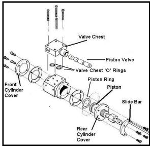
Piston valve cylinder assembly.
