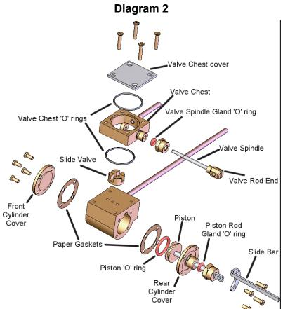
Round slide valve cylinder assembly. First introduced in 1999 on the 'basic series' locomotives gradually but phased in on 'classic series' models from 2002. There are several variations of this, some with sloping or smaller 3/4" square valve chests, but all are essentially of similar construction.
