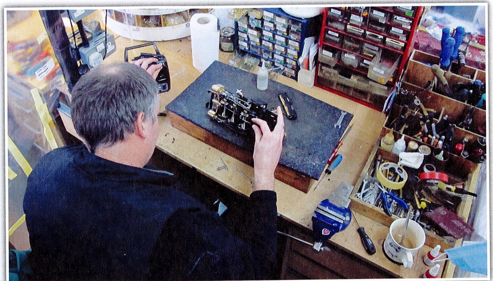
Once run-in, the chassis moves on to assembly, where everything needed to make the locomotive run is added, including radio control (80% of models sold are fitted with RC).
