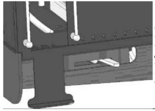
On a manually operated Silver Lady, the lever to operate the Dummy Drain cocks / Exhaust Valve, protrudes through the chassis frame, under the Right Hand cab floor. The drawing opposite shows the valve set for 'Exhaust'.
