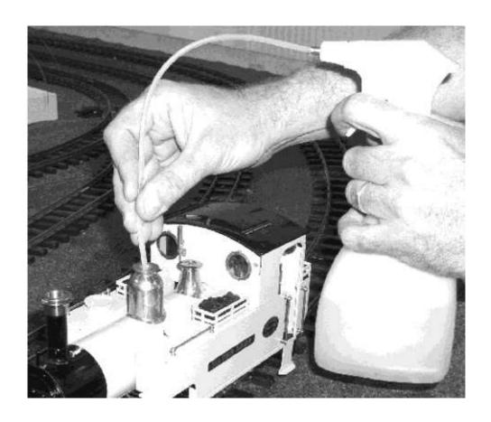
You will sometimes see water and air bubbles passing through the sight glass as you pump so allow the level to settle after a few pumps. Carefully pull the plastic pipe out of the water filling valve whilst steadying the engine.
