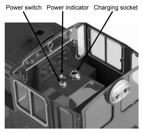
It will initially take approximately 5 hours for the batteries to fully charge. The time taken for subsequent full charges may be less. When the batteries are fully charged, the LED will change to green. The charging jack should now be removed from the locomotive and the charger unplugged from the mains.
