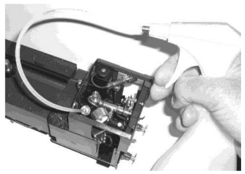
Push the end of the plastic tube into the socket in the top of the water filling valve.
