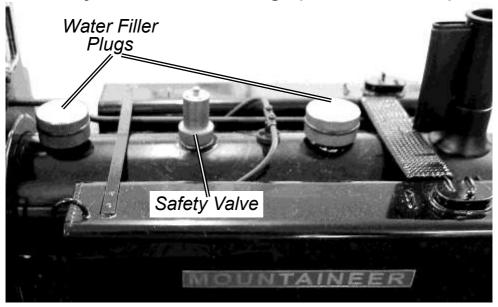
There has to be a space above the water to allow steam to be raised so, insert the end of the plastic pipe into the boiler and withdraw 30 ml of water with the syringe. Replace the filler plug finger tight, and then place the dome back over it. Note that there is a rubber 'O' ring around the body of each filler plug. This is to retain the domes during normal operation.
