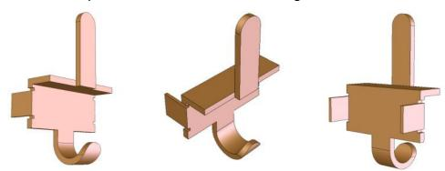
Folding the Lamp Brackets - three angles of the same Lamp Bracket are shown here for clarity.
