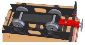
frames, and another M3 x 6 screw to fix the centre buffer to the rear frame spacer.
