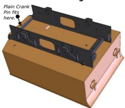
Turn the Tender Body and slide the front spacer of the assembled frames and slide it under the bracket at the front of the Tender body. Use two M3 screws from inside the Tender body to fasten the rear frame spacer to the Tender. Now fit the Plain Crank Pin through the bracket into the centre hole of the front frame spacer. Use a small pair of pliers to tighten this up.
