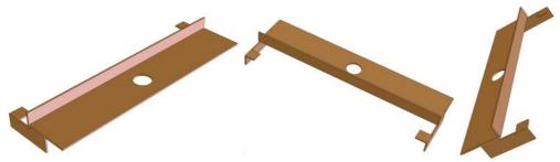
Folding the Tender Back Plate - three angles of the same plate are shown here for clarity.
