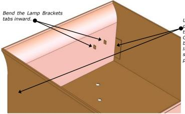
Use clamps at these points to hold the rear of the Tender in place. Check that all is square before soldering. If not, loosen the clamps slightly and adjust the position.
