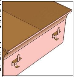
Rear of the Tender, showing the position of the Lamp Brackets.
