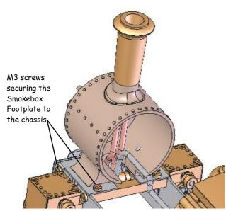
rear of the steel footplate is fixed to the frame spacer, again using 2 x M3 brass CH screws. The centre hole of this frame spacer is not used.
