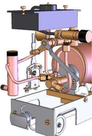
drain facing you, the left hand pipe bends up and inwards to connect to the the regulator and right hand pipe bends down and round the back of the lubricator to connect to the end of the superheater pipe where it emerges from the flue tube.
