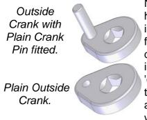
Now convention says that the right hand side should lead. All this means is that when the model is running forward, the right hand crank is 90 degrees, or a quarter of a revolution in front of the left; hence the term 'quartering'. We always observe this, though it would make no difference at all to the running if it were the other way round.
